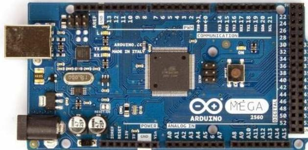
**Gambar 2.5.** Arduino Mega[13]
