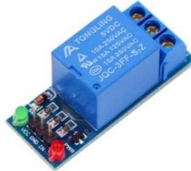
**Gambar 2.18.** Modul Relay 1 Channel[22]
