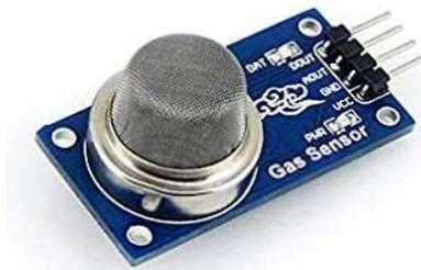
**Gambar 2.15.** Sensor Gas MQ2[15]
