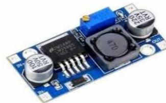
Gambar 11. Modul *Step Down DC-DC*[20]
