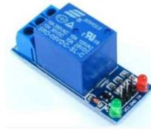
Gambar 9. Modul *Relay 1 channel*[19]
