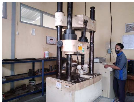
Gambar.3.2 Alat Uji Tarik Universal Testing Machine . (Dokumentasi,2021)
