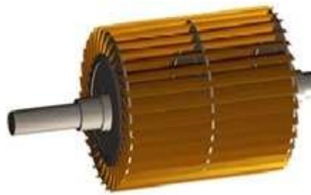
Gambar 2.2 Turbin Cross flow
