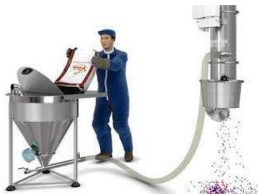
Gambar 2.14 Pneumatic Conveyor (Pengadaan.web.id, 2021)
