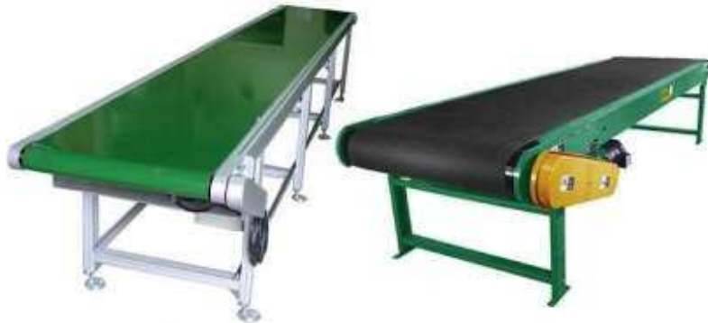
Gambar 2.11 Belt Conveyor (Pengadaan.web.id, 2021)
