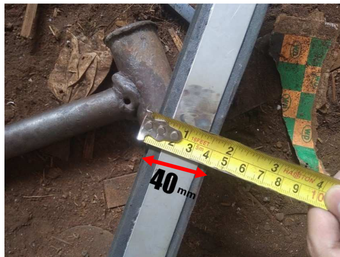
Gambar 4.18 Pengecekan Dimensi Rubber Lebar 40 mm
