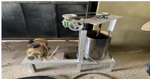
Gambar 4. Bagian detail Mesin *Injection Molding* ( Abdurokhman, 2012 )
