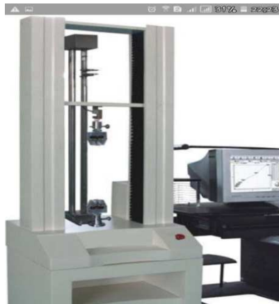
Gambar 2. 1 alat uji tarik ununiversal testing
