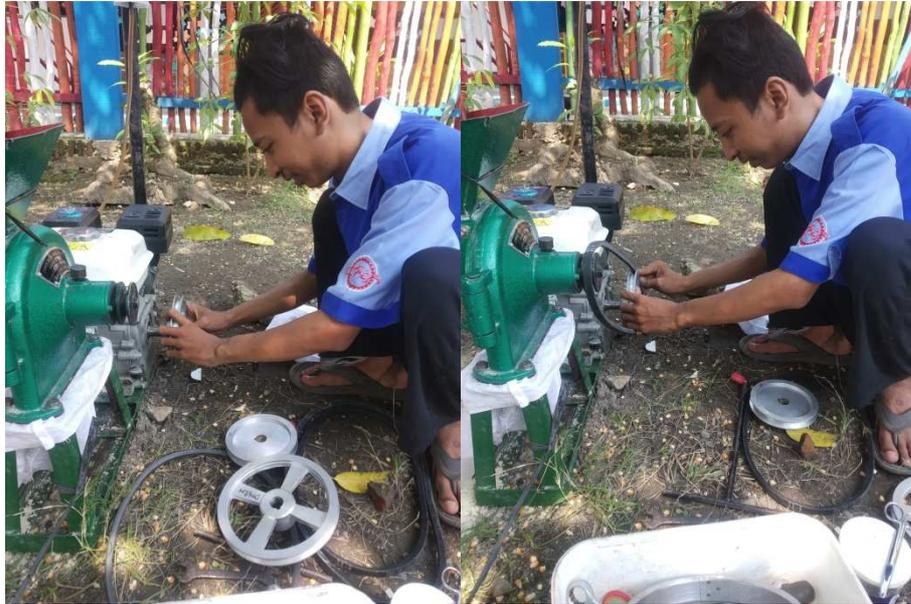
Gambar 3. 12 Pemasangan Puli 7 inch Dan Sabuk V
