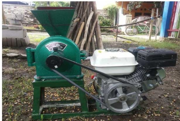
Gambar 2. 1 Mesin *Disc Mill* FFC 15
