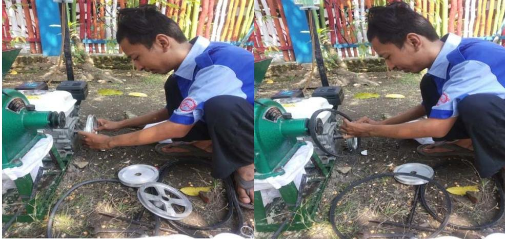
Gambar 3. 10 Pemasangan Puli 5 inch Dan Sabuk V
