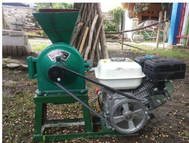
Gambar 3. 17 Mesin *Disc Mill* FFC 15
