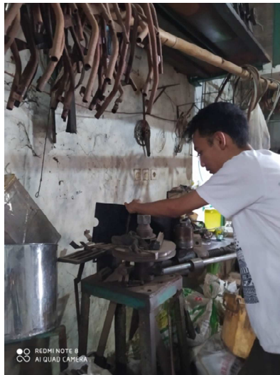
Gambar 4.4 Proses Pembengkokan Plat Stainless steel 304
