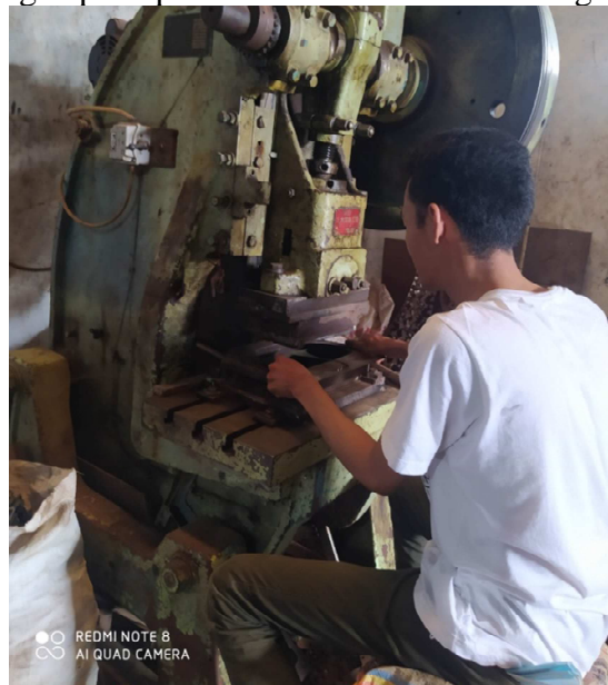
Gambar 4.2 Proses pemotongan plat Stainless steel 304
