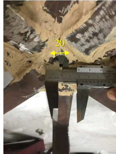
Gambar 4.18 Diameter Lubang Baut
