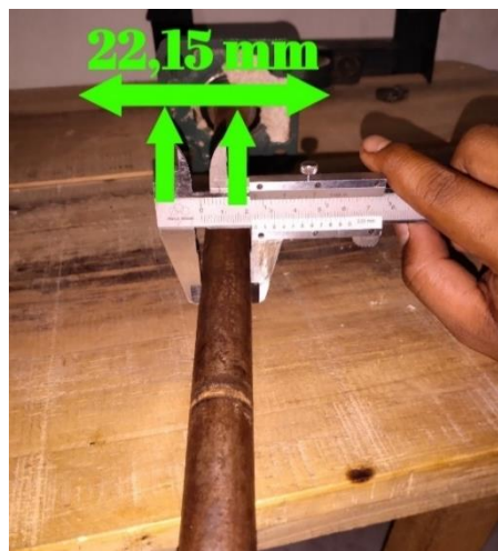
Gambar 4. 53 Diameter besi poros bearing duduk
