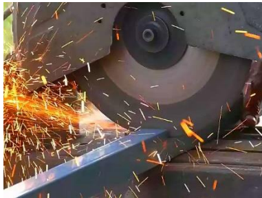
Gambar 4. Pemotongan Stainless Steel Siku
