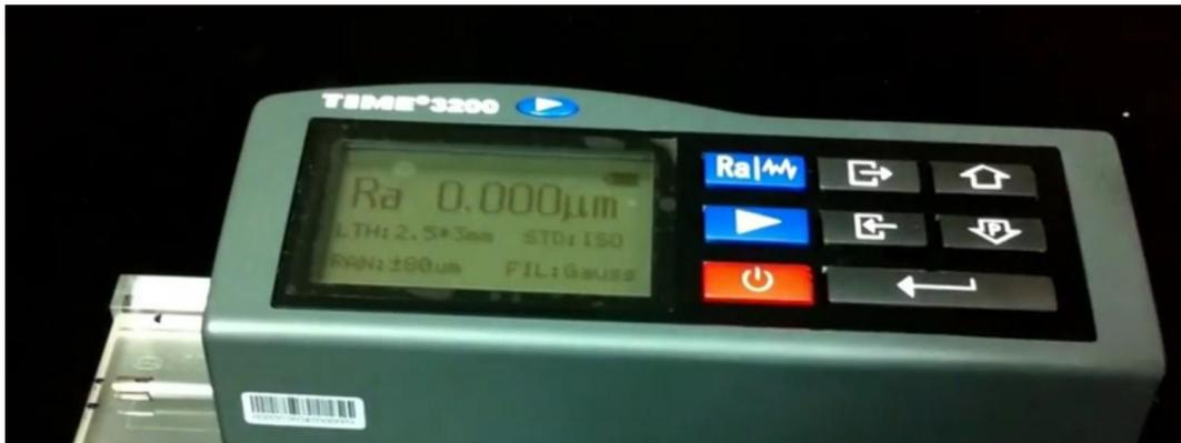
Gambar 2.3 *Surface Roughness Tester Type TIME3200*
