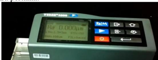
Gambar 3. Surface Roughness Tester Type TIME3200
