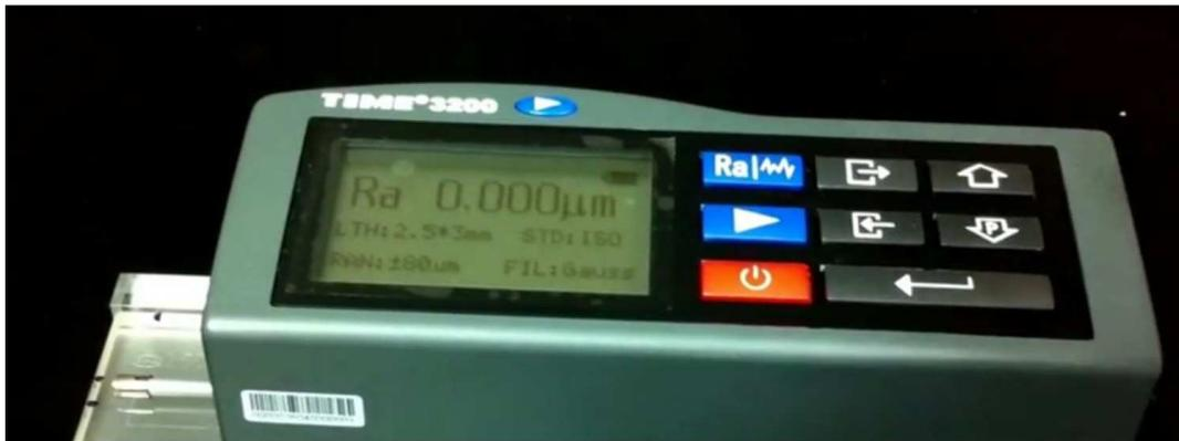
Gambar 2.3 *Surface Roughness Tester Type TIME3200*
