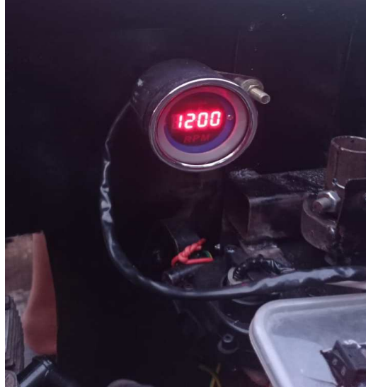
Gambar 3.5 Tachometer digital (Dokumentasi, 2021)
