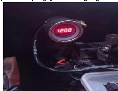
Gambar 3.4 Tachometer digital
