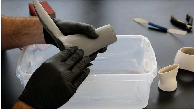
Gambar 2. 22 Proses finishing objek 3D print
