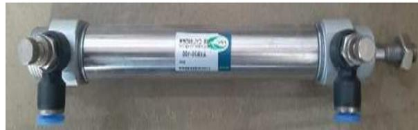
Gambar 3.17 *Cylinder Double Acting*
