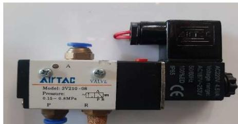
Gambar 3.19 *Solenoid 3/2 Valve 220 VAC*
