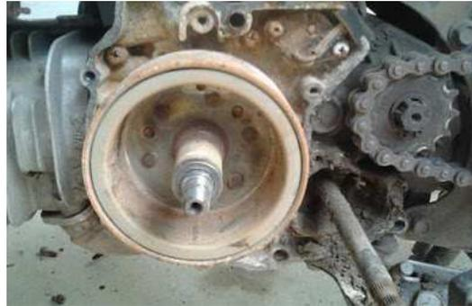
Gambar 2.6 Rotor Magnet
