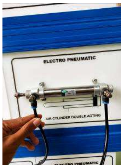
Gambar 4.32 Cylinder double acting bergerak mundur (dokumentasi, 2021)
