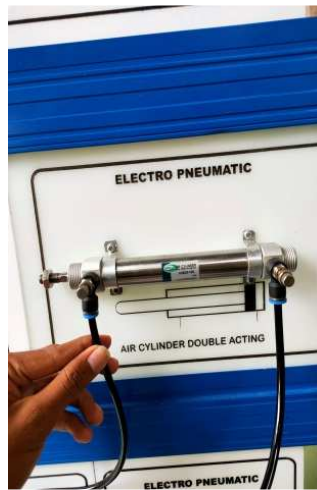
Gambar 3.7 Cylinder double acting (Shiddiq, 2018)
