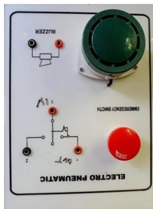
Gambar 4.4 buzzer dan emergency switch
