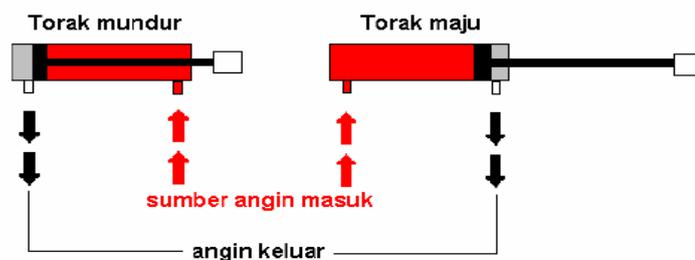
Gambar 2.7 Silinder kerja ganda (*Double Acting Cylinder*)
