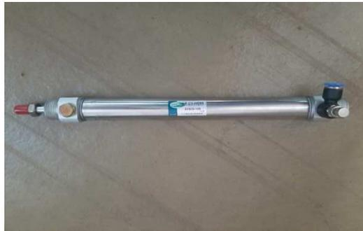
Gambar 3.11 Tampilan *Cylinder Single Acting*
