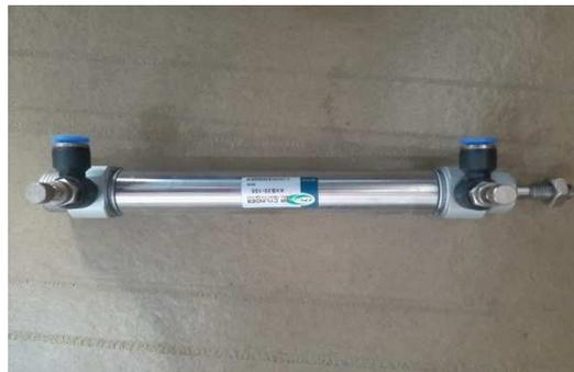
Gambar 3.12 Tampilan *Cylinder Double Acting*
