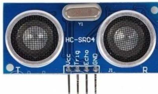
Gambar 2.1 Sensor Ultrasonik HC-SR04
