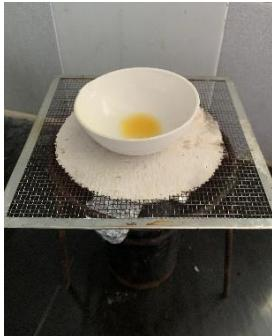
A photograph of a white bowl containing a small amount of yellow oil (lanolin) sitting on a metal mesh over a heat source, likely being melted.                                                                                                                                                          | Memanaskan zat pengikat lanolin sampai mencair |
