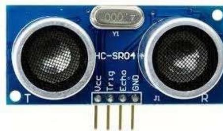
Gambar 2. 8 Sensor Ultrasonik
