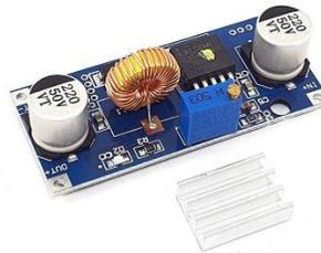
Gambar 2. 11 Modul Step-Down DC to DC 5A XL 4015
