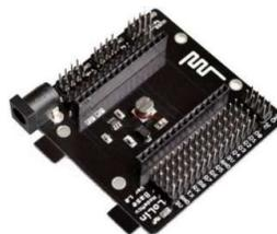
Gambar 2. 7 NodeMCU ESP8266 Base Board
