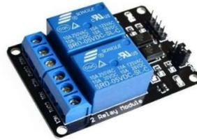
Gambar 2. 9 Relay 2 Channel
