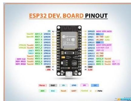
Gambar 2. 5 *PinOut ESP32*
