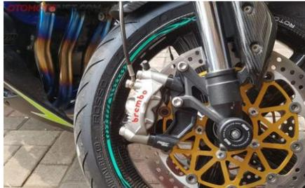
Gambar 2.11 Rem cakram *double piston* (Industry, 2020).
