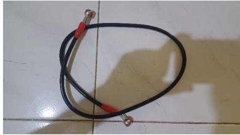
Gambar 2.7 Kabel/selang rem
