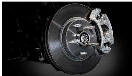
Gambar 2.10 Rem hidrolik (Wuling, 2024).
