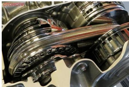
Gambar 2.18 Transmisi Otomatis CVT
