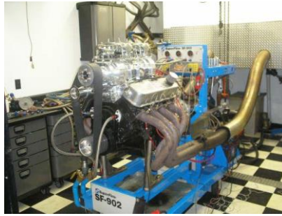
Gambar 2. 6 Engine Dynotets (Cinta Mobil.com, 2019)
