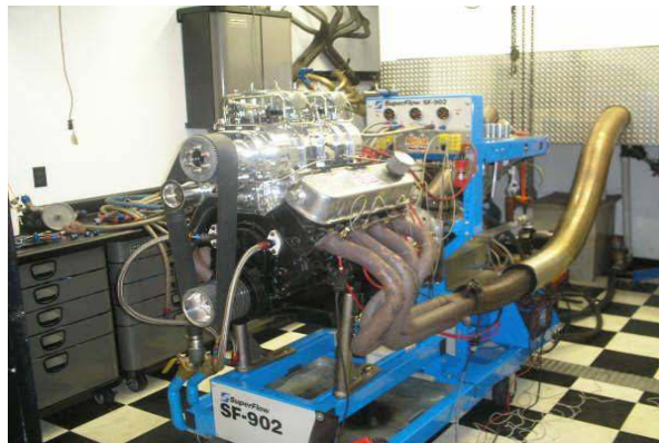
Gambar 2.4 Engine Dynotest (Mobil, 2019)
