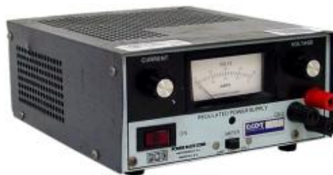
Gambar 2.4 Power Supply (cahyokrisma,2010)
