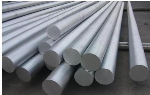
Gambar 2.12 Aluminium Magnesium Silikon *Alloy*
