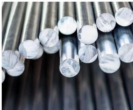
Gambar 2.12 Aluminium Magnesium Silikon Alloy
