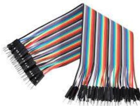
Gambar 2. 7 Kabel Jumper
