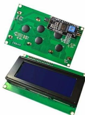
Gambar 2. 8 LCD 20 X 4
