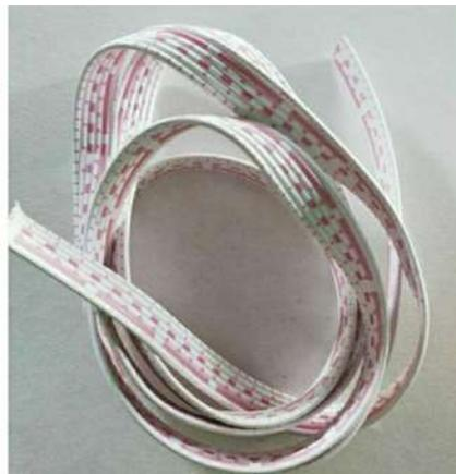
Gambar 2. 14 Kabel Flat 6 Pin
