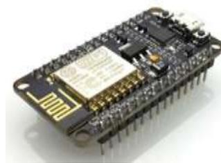
Gambar 2. 2 *NODEMCU ESP8266*
