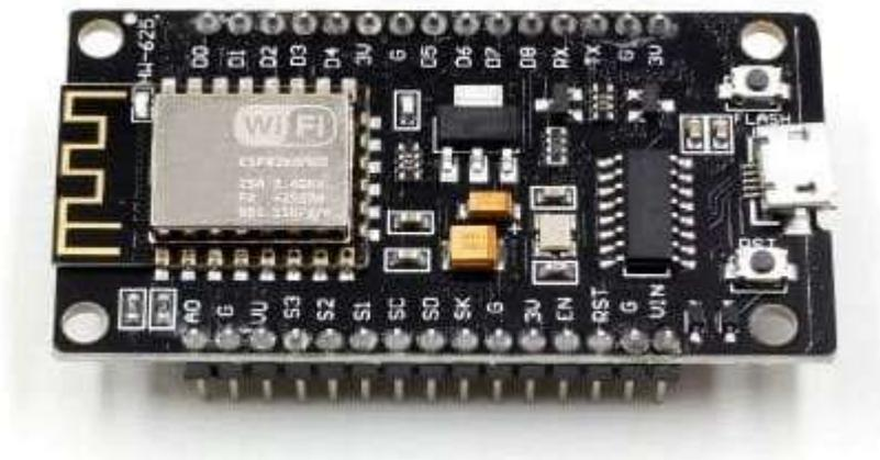
Gambar 2.2 NodeMCU ESP8266
