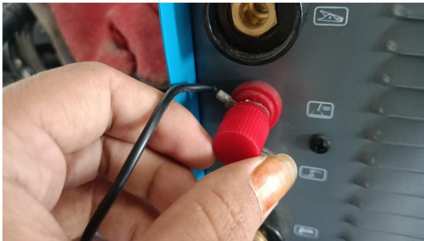
Gambar 3. 16 Memasang Kabel *Grounding*
