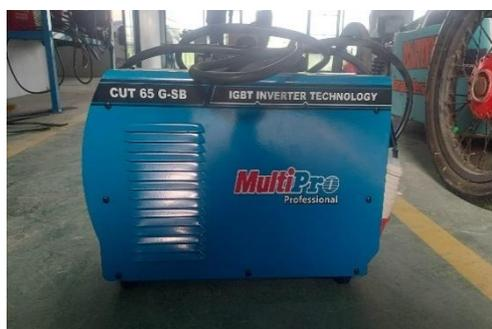
Gambar 3. 2 Mesin Plasma *Cutting*
