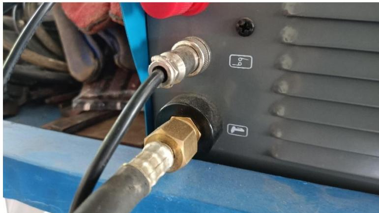
Gambar 3. 18 Memasang Kabel *Gas Electric Connector*
