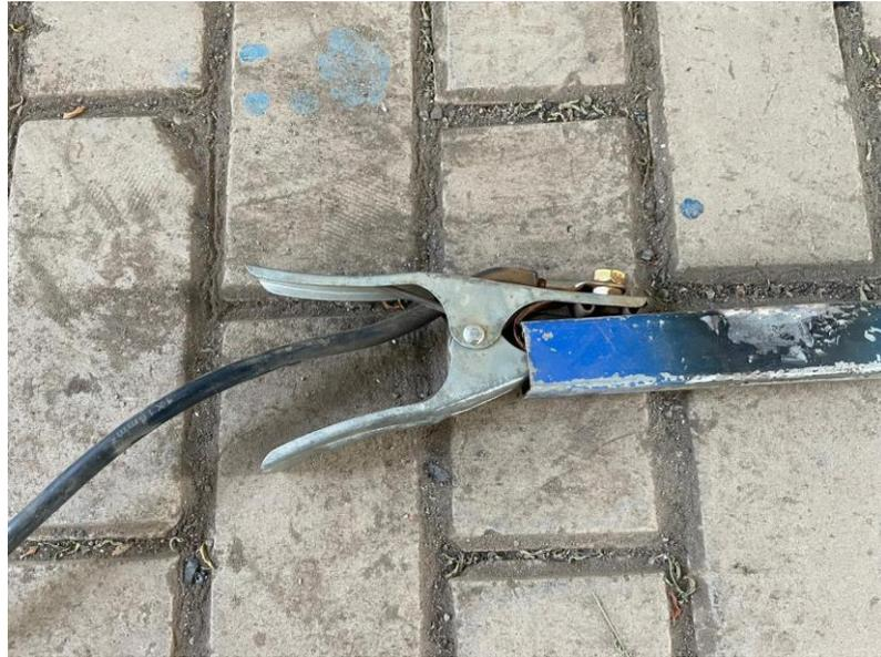
Gambar 3. 22 Memasang *Clamp* Kabel Massa
