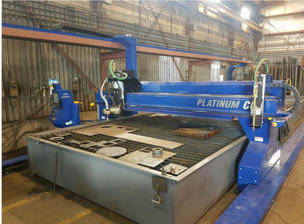
Gambar 2. 8 CNC Plasma Cutting (Modernmachinery, 2024)
