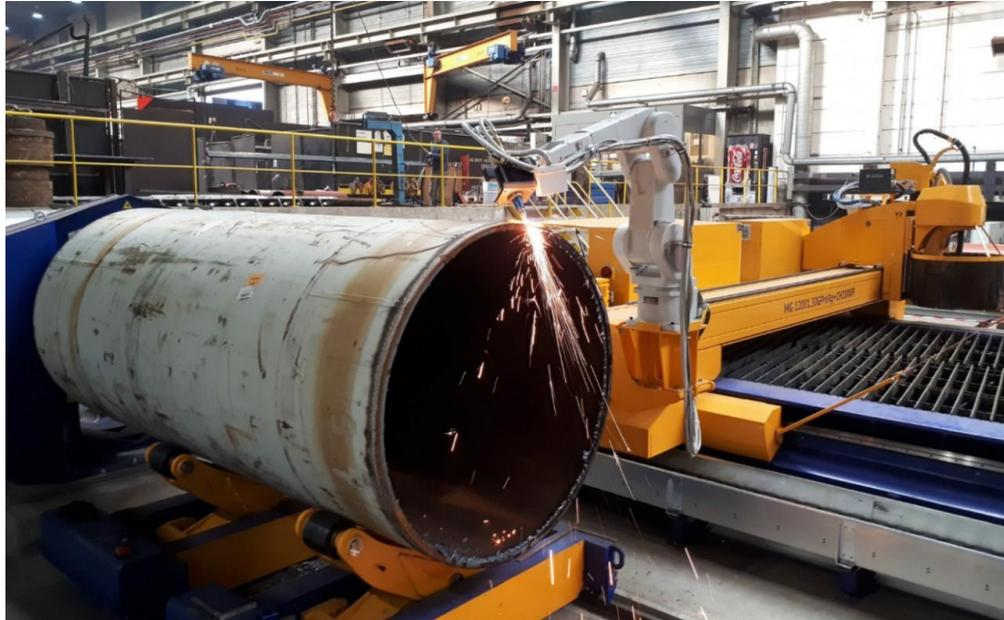
Gambar 2. 9 Robotic Plasma Cutting (Robotmaster, 2024)
