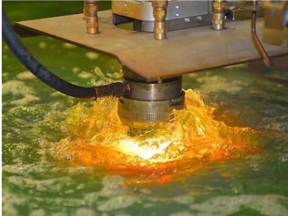
Gambar 2. 6 *Underwater Plasma Cutting* (ESAB, 2024)
