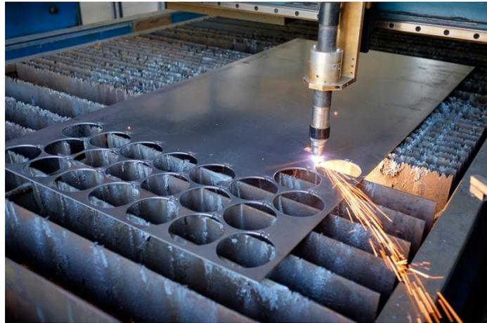
Gambar 2. 1 Plasma *Cutting* (Fractory, 2021)
