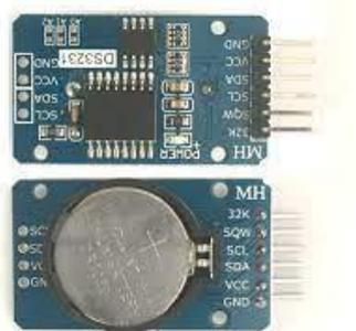
Gambar 2. 4 RTC (*Real Time Clock*)
