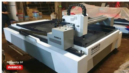
Gambar 2.6 *Plasma Cutting CNC*
