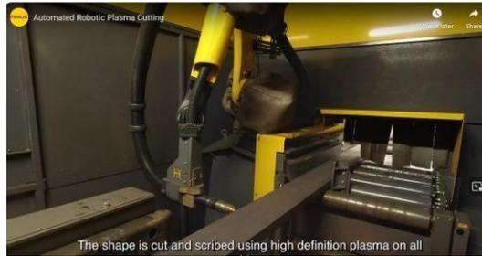
Gambar 2.7 *Robotic plasma cutting*
