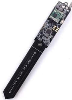
Gambar 2 . 7 *Soil Moisture Sensor V3*
