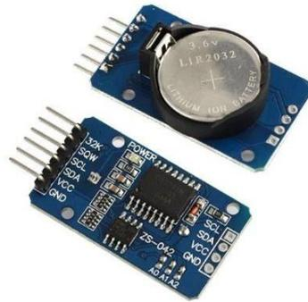
Gambar 2. 8 RTC (REAL TIME CLOCK) Sensor
