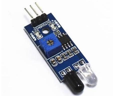
Gambar 2.7 *Infrared Barrier Obstacle Sensor*
