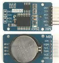
Gambar 2.9 RTC (*Real Time Clock*) Ds3231
