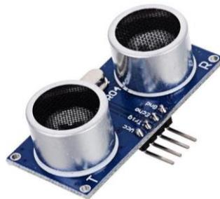
Gambar 2.6 Sensor Ultrasonik
