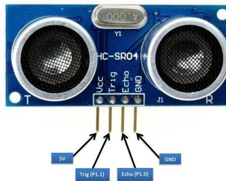
Gambar 2. 1 Sensor Ultrasonik
