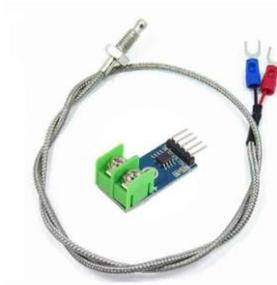
Gambar 2.4 *Thermocouple* MAX6675
