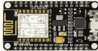
Gambar 2.1 NodeMCU ESP8266
