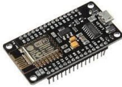
Gambar 2.6 NodeMCU
