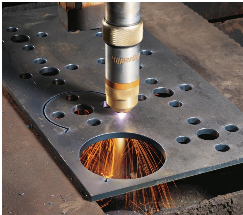
Gambar 2.3 Water Injection Plasma Cut(westermans, 2013)
