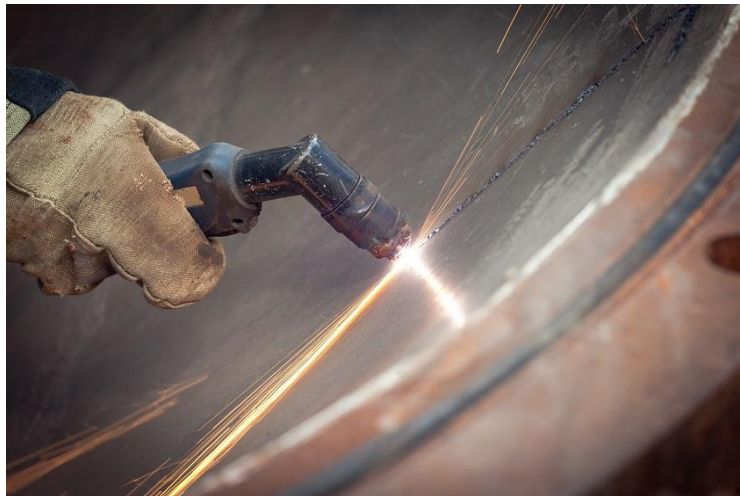
Gambar 2.4 Dual Gas Plasma Cutting
