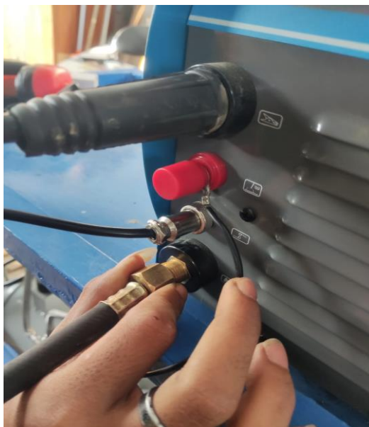
Gambar 3.16 Pemasangan kabel gas electric connector
